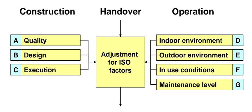
$ESL = RSL \times A \times B \times C \times D \times E \times F \times G$
